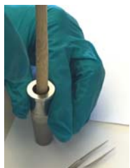
3. Press Edges Down with Rod
