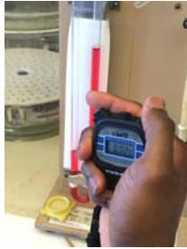
5. Start Timer when Liquid Reaches Next Mark Down from Top (2 nd Mark)
