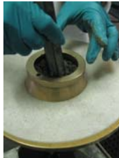
2. Tamp 20 Times. Incline Tamper when Near Perimeter.
