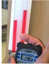
6. Stop Timer when Liquid Reaches Next Mark Down from Top (3 rd mark)
