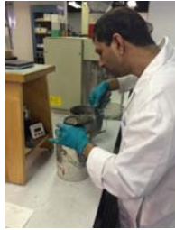
5. Slice Off Excessive Paste
