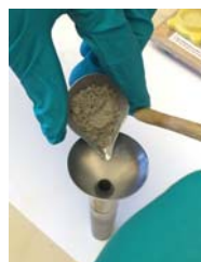
5. Place Cement Sample in Cell
