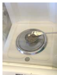
4. Measure Cement Mass to Nearest 0.001g
